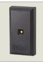
Farpointe Data mullion mount Indala format proximity surface mount reader. Wiegand output. Reads the Keyscan 125 kHz 36-bit Indala format. A HID PX-603 replacement reader. Black. 18" (457.2 mm) – 9 conductor shielded cable pigtail. Two-piece design with snap-on cover to hide mounting screws. Weight is 3 oz (85 g). Product Listings: UL294, FCC, IC. Warranty: Limited
