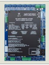
The Keyscan CA250B is a access control panel only. It is available to replace non-functioning CA250 access control panels.
