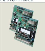
When circumstances dictate a long cable run between control panel and reader, exceeding 500 feet, rely on the Keyscan WIEEX2 wiegand extender. This interface converts the Wiegand signal to standard RS485 providing a communication range of up to 4000 feet between WIEEX2 receiver and WIEEX2 transmitter while using standard CAT5 cable between units.
