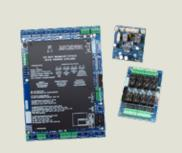
The Keyscan CA250NBM is a network appliance-based access control unit that gives you unmatched flexibility for new installations or revitalizing aged or failing access control systems. The CA250NBM is a package that includes 1 CA250B ACU board, 1-OCB8 relay board, and 1-DPS-15 power supply. This hardware is programmed for up to 90,000 credentials. This does not include a black metal enclosure.
