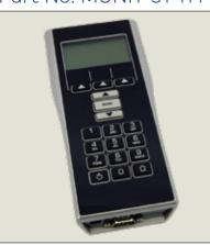
The M-Unit is a diagnostic and configuration data transfer tool designed to be used with E-Plex locks. It allows programming of offline E-Plex locks by gathering data from Aurora/LUNA software and transferring it the lock. It can also transfer audit trails and be used as a site survey tool for efficient placements for E-Plex wireless lock systems.
