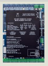
The Keyscan EC1500B is an elevator floor access control panel only. It is available to replace non-functioning EC1500 access control panels.
