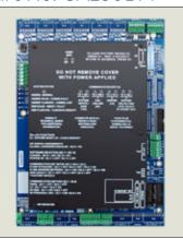
The Keyscan CA250BM is a access control panel only. It is available to replace non-functioning CA250M access control panels.
