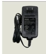
The PS1225 is a replacement 12VDC plug-in switching transformer for the SDACSKT (SDAC Kit). Plugs into standard 120 Vac outlet and provides up to 2.5 amps. Has 60" of 18 Gauge cable for mounting close to SDAC control. Has 2.1 mm barrel power connector. Center positive. For replacement of transformer provided in the SDACSKT. C/UL/US Listed Black Colour
