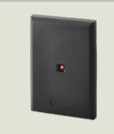
Farpointe Data single-gang mount Indala format proximity surface mount reader. Wiegand output. Reads the Keyscan 125 kHz 36-bit Indala format. A HID PX-605 replacement reader. Black. 18" (457.2 mm) – 9 conductor shielded cable pigtail. Two-piece design with snap-on cover to hide mounting screws. Weight is 4 oz (113 g). Product Listings: UL294, FCC, IC. Warranty: Limited Lifetime.
