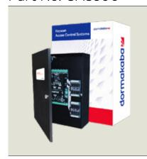
The Keyscan CA8500 is a network appliance-based access control unit that gives you unmatched flexibility for new installations or revitalizing aged or failing access control systems. The CA8500 is a package that includes 1 CA8500B ACU board, 2-OCB8 relay boards, 1-DPS-15 power supply, and 1-black metal enclosure with lock and tamper switch.
