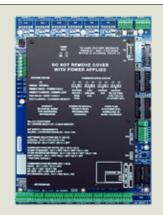
The Keyscan EC2500BM is an elevator floor access control panel only. It is available to replace non-functioning EC2500M access control panels.
