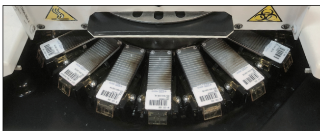
Figure 1. Specimen section placed on Trajan Series 3 Adhesive microscope slides on an automated immunostainer
