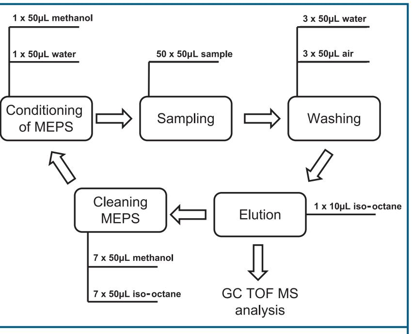
Figure 1: Schematic view of the MEPS sample preparation process in analysis of sewage water.
