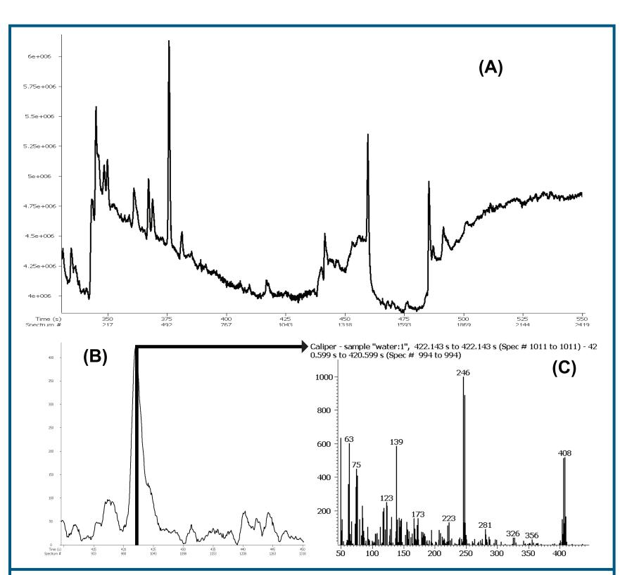
Figure 3: MEPS-GC TOF MS analysis of sewage water sample. (A) TIC chromatogram of sewage water. (B) Zoomed part of chromatogram – masses 406+408 are displayed. (C) Measured mass spectrum of natively present BDE-28
