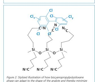
The cyanopropyl chains allow the cyano groups to adapt to the shape of individual analytes (for example a PCB shown in Figure 2). Such adaptive chemistry presents a very low steric barrier to analyte-phase interactions.
