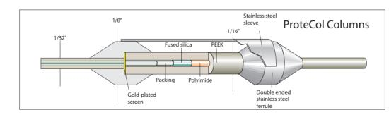
Standard Column Length: 50, 100 or 150mm Frit design: deactivated gold-plated woven stainless steel mesh 140µm thickness Standard IDs: 75, 150, 300 or 530 μm
