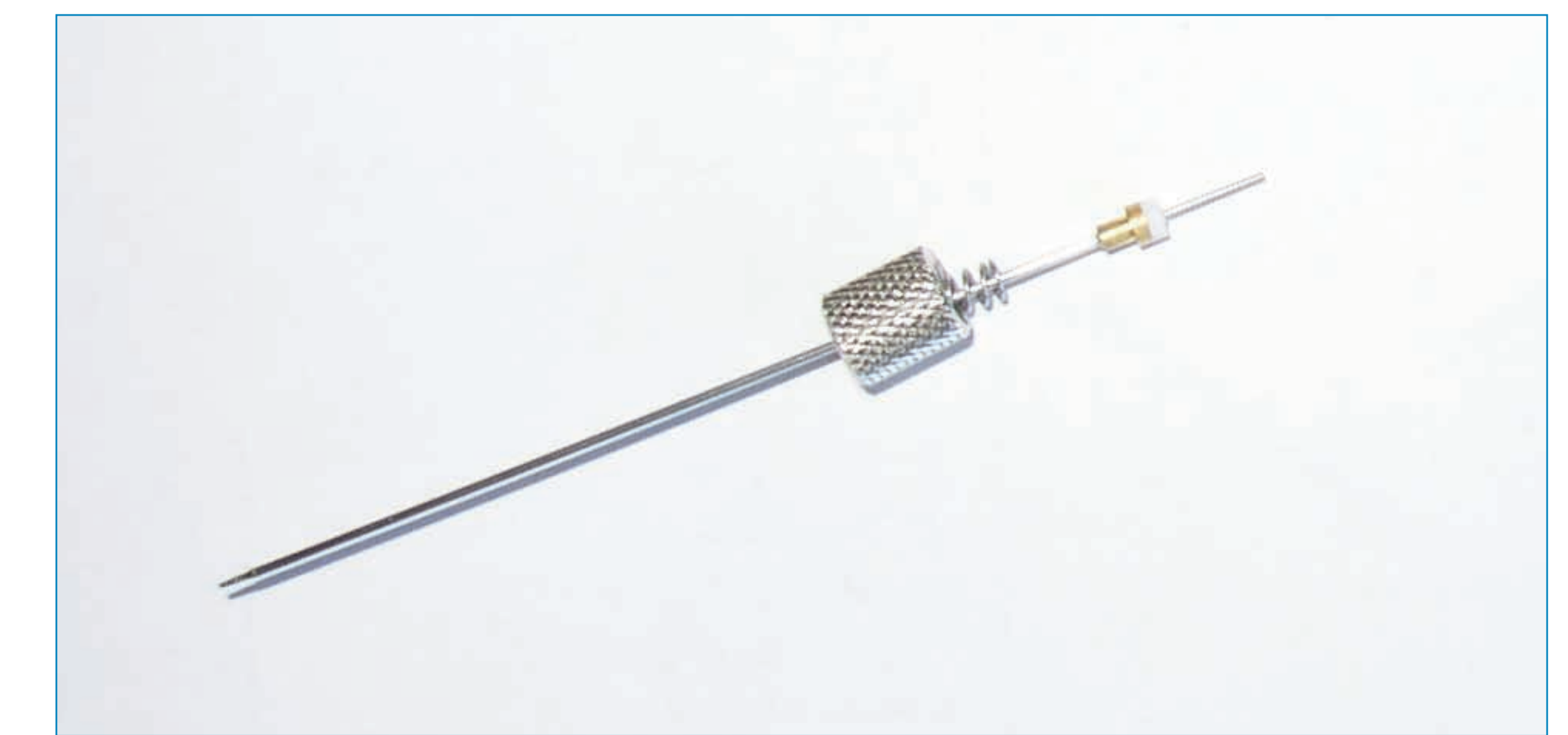
Figure 4. A picture of the iLPE needle ready to be fitted to a gas-tight GC syringe
