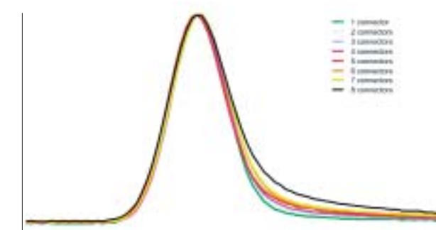
Figure 8. Effect of the number of connections on peak broadening
