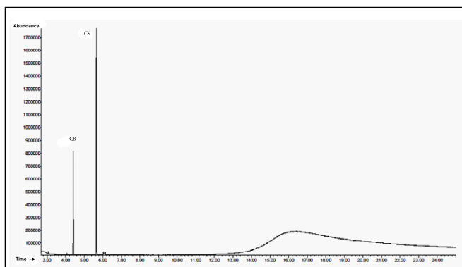
Figure 9. Alkane test mix response on MS backflush initiated at 6 minutes.
