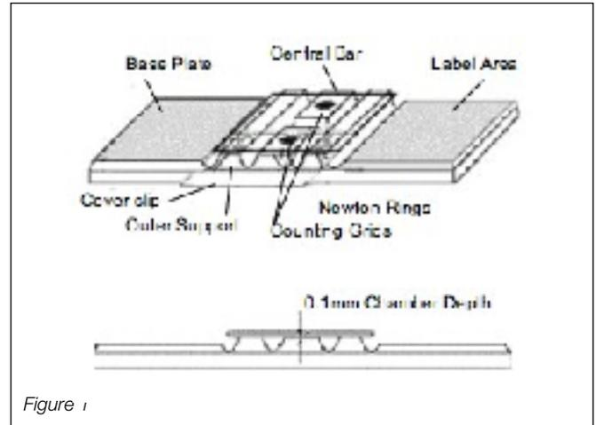
This bar is deeper in relation to the outer supports, typically by 0.1 or 0.2 mm.
