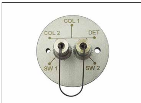
Figure 1. SilFlow Deans' switch
