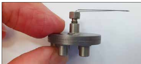
Figure 8. The standard 66 mm restrictor attached to the SilFlow device.
