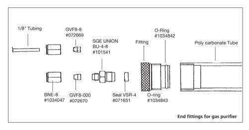
SGE gas purifiers are designed to remove harmfull impurities from gas streams, although, because they are constructed of polycarbonate, they are not recommended for use in the clean up of carrier gas in capillary gas chromatography.
