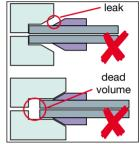
Figure 2. Stainless steel ferrules do not adjust for different manufacturers fittings leading to leaks or dead volume
