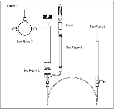
1. Remove the existing packed column from the instrument. If 1/8" O.D. packed columns are being used, the 1/8" adaptors should be removed to accommodate the larger CCS capillary injector and detector fittings.
