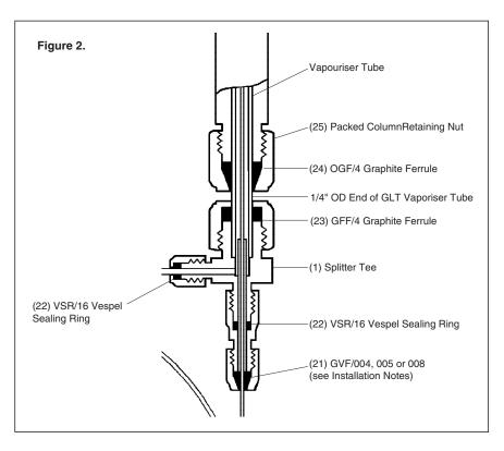
One end of this tube is bushed up to 1/4" O.D. The split tee (1) is connected to the 1/4" section.
