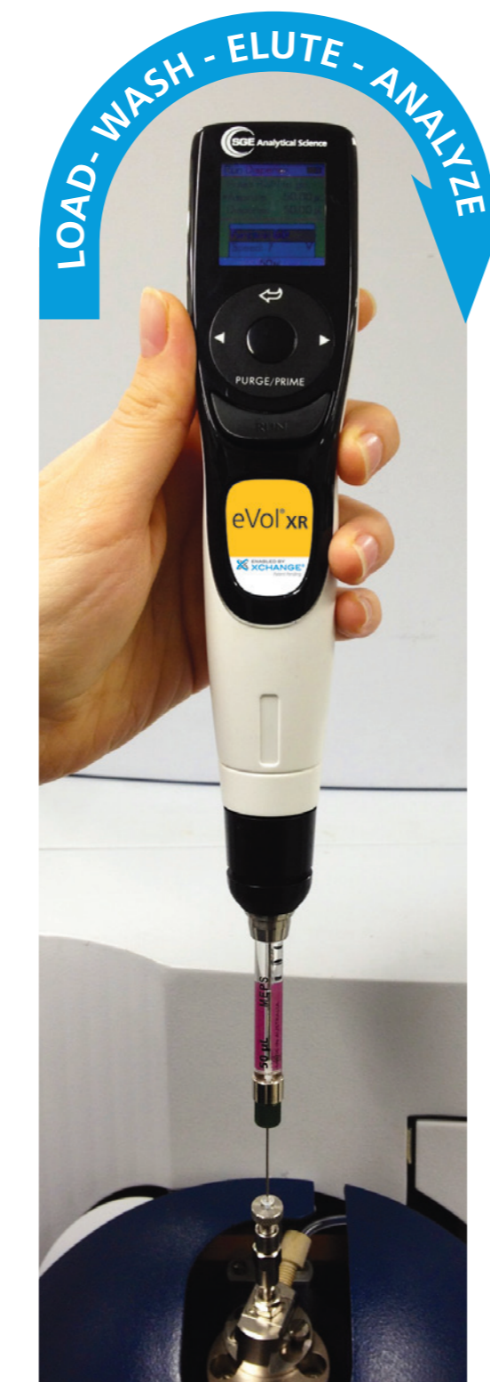
Figure 3. eVo ® MEPS: a programmable digital syringe with embedded SPE capability
