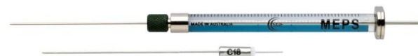
Figure 1. The MEPS™ syringe and SPE cartridge or BIN “ B arrel I nset and N eedle” filled with 2 mg of sorbent commonly used for SPE.
