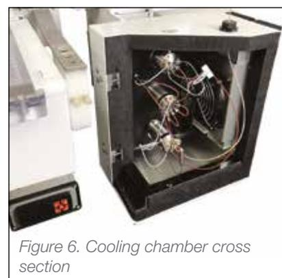
Figure 6. Cooling chamber cross section
