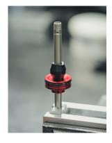
Apply fresh red Loctite to the shaft thread and thread the Luftkappe stud into place by hand.
