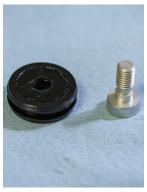
Separate Luftkappe dome from its piston (unthread by hand).
