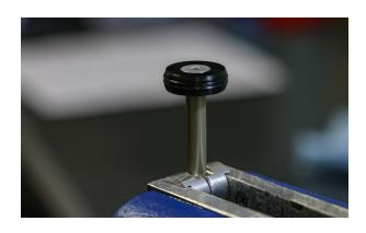
Use a 4mm allen key to undo the silver piston bolt and remove the piston from the shaft.
