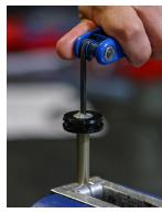
Remove the o-ring from behind the threads of the piston bolt and discard.
