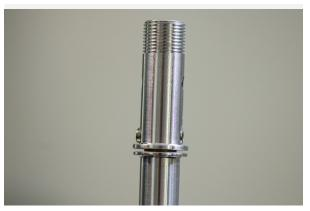
Slide the plastic Luftkappe piston onto the stud, lining up the slots in the piston with the roll pin.
