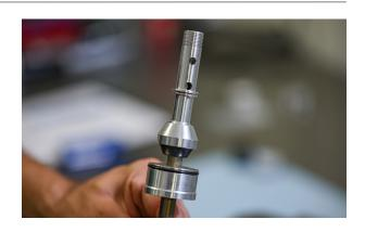
Compress the new roll pin (using vise, knipex or multigrips) to get it started in the hole, then press it all the way in the vise. It does not need to be centered, but needs to be through both holes.
