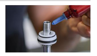
Thread dome on to piston by hand, and torque to 50in.lbs (5.5Nm).
