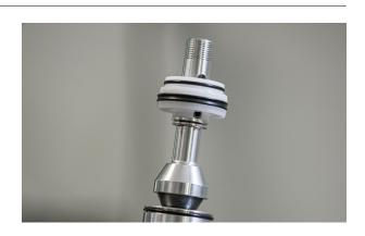
Lubricate o-ring on piston, and inside of Luftkappe dome where it will contact the o-ring.
