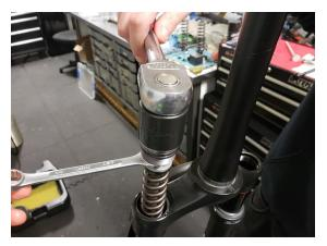
8. Use a Torque wrench + 28mm chamferless socket on the TOPCAP and a 12mm Spanner on the SPRING COLLAR to torque to 45in.lbs without loctite. DO NOT EXCEED TORQUE SPECIFICATION.
