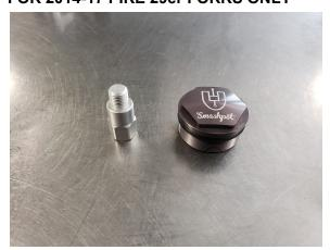
13. All PIKE kits include a 20 mm long TOPCAP ADAPTOR to be used when installing the kit in a (2014-17) 29in fork. All 27.5in PIKES and 29in PIKES from 2018 onwards do not require this adaptor.
