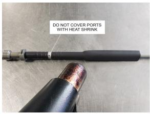
5. Position and install the included length of HEAT SHRINK just shy of the ports and extending over the end of the SEAL HEAD using a heat gun. \*\*Make sure you do not cover the ports with Heat Shrink
