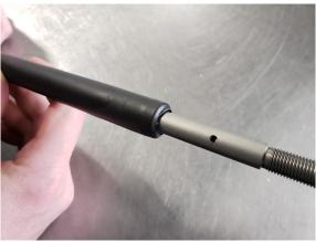
6. Push INNER TUBE into the OUTER TUBE assembly as far as possible. Using a sharp knife or scissors, trim back the Heat Shrink to be in line with the end of the Seal Head. (Try not to score the shaft with the knife but note that scratches are not critical it is not a sealing surface.)
