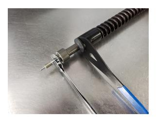
2. Use a 22mm Cone Wrench on the BOTTOM OUT CONE and a 12mm Spanner on the FOOTSTUD to remove the FOOTSTUD and shim stack assembly from the rest of the OUTER TUBE ASSEMBLY.
