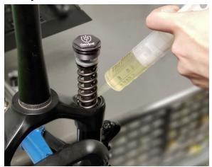
25. Using a syringe or graduated cylinder add 20wt suspension fluid as per the following table.
