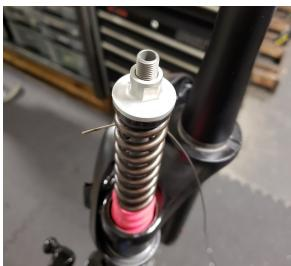
6. Install the SPRING PERCH and SPRING COLLAR onto the INNER TUBE and tighten down until 8-10mm of threads are exposed.
