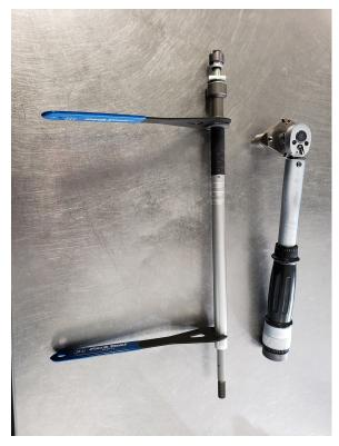
4. Using a 14mm cone wrench on the SEAL HEAD and a 22mm cone wrench on the BOTTOM OUT CUP - use a Torque wrench to torque SEAL HEAD to 75in.lbs without loctite.
