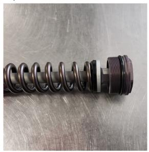
15. Thread the TOPCAP onto the INNER SHAFT ASSEMBLY
