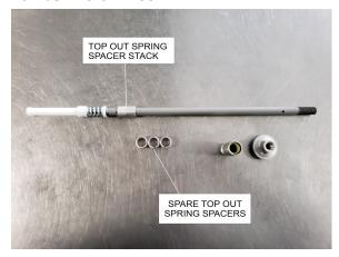
2. Install a stack height of TOP OUT SPRING SPACERS as required to suit your fork travel. TOP OUT SPRING SPACERS must sit on the INNER TUBE between TOP OUT SPRING ASSEMBLY and SEALHEAD. See Drawing 2 and table below for details. For example: a 160mm travel fork requires 20mm of TOP OUT SPRING SPACERS so install 2 x 10mm spacers.
