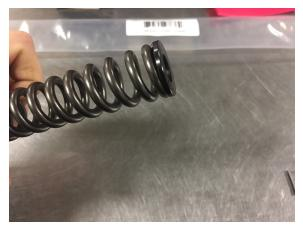
8. Place the acetal SPRING PERCH into the end of the COIL SPRING. It may fit one end of the spring better than the other. The better fitting end will be the top of the spring as oriented in the fork.
