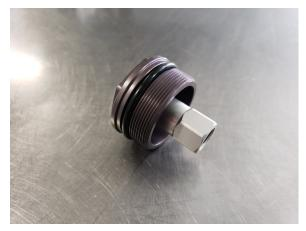
14. Thread the TOP CAP ADAPTOR into the TOPCAP. Use a Torque wrench, 28mm chamferless socket and 13mm Spanner to torque to **45in.lbs** without loctite.
