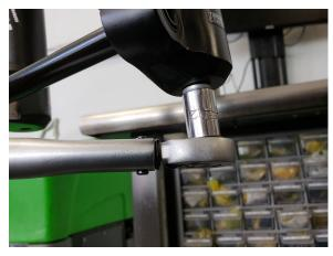
23. Use a Torque wrench and 12mm socket to torque the FOOTNUT to 55in.lbs without loctite.
