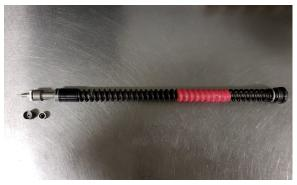
20. The complete Smashpot assembly is now ready to be inserted into your fork and should look like the picture above.
