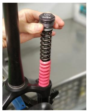
21. Apply a generous amount of Slick Honey grease to the COIL SPRING especially the portion covered in Heat Shrink. Insert assembly into the fork as shown. Be careful as the needle adjuster is small diameter and could be damaged if the assembly is dropped into the fork lower.
