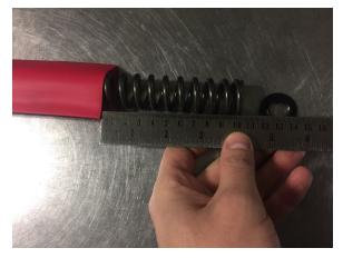
9. Slide the Heat Shrink provided on to the COIL SPRING, approximately 100mm from the top end of the spring where the SPRING PERCH will be fitted.
