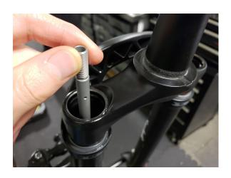
3. Remove SPRING COLLAR, SPRING PERCH and COIL SPRING. The INNER TUBE will fall down inside the stanchion. Compress the fork fully and you should be able to grab the INNER TUBE and pull it out of the stanchion.
