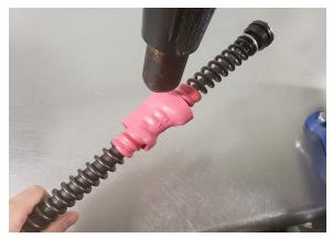
19. Using a Heat Gun, install additional 50mm length of red Heat Shrink over the top of existing Heat Shrink on the COIL SPRING. This step helps prevent noise from spring deflection due to the larger diameter stanchion on the Fox 36. NOTE: NOT NECESSARY ON 36 RHYTHM.
