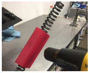
10. Use a heat gun to heat the Heat Shrink until it fits snugly over the COIL SPRING. Once shrunk, trim any excess from the ends of the Heat Shrink that protrudes inside the inner diameter of the COIL SPRING. When complete, check that the spring slides smoothly over the cartridge OUTER TUBE.
