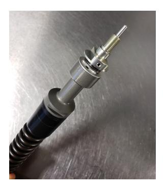
4. Reinstall the FOOTSTUD and modified shim stack into the OUTER TUBE ASSEMBLY.
