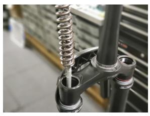
5. Use the shift cable to pull the INNER TUBE up through the COIL SPRING until the threads of the INNER TUBE are exposed above the COIL SPRING.
