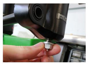
22. Install CRUSH WASHER and FOOTNUT onto the FOOTSTUD.
