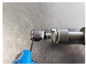
17. If the ADJUSTER DIAL and footnut are installed already on your FOOT STUD, use a 1.5mm allen key to unscrew the set screw in the ADJUSTER DIAL until it slides easily off.
