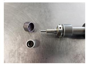
18. Unscrew the FOOTNUT by hand and remove it and the CRUSH WASHER from the assembly.
