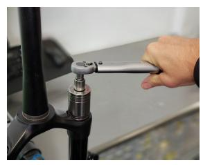
26. Use a Torque wrench and 28mm chamferless socket to torque the TOPCAP to 220in.lbs (for FOX) 250in.lbs (for ROCKSHOX) without loctite.
