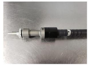
7. Install a stack height of MAIN SPRING SPACERS on the outer tube as required to suit your fork travel. See Drawing 2 above
