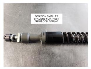
12. Check that the COIL SPRING is adequately pre-loaded so that it is not able to rattle around. One or two of the 2mm SPRING SPACERS (part number: 13-07-3-08) may be required for appropriate preload. Position the longest spacers closest to the COIL SPRING and the shortest spacers furthest away as this help stabilise the spring assembly during use.
