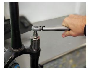
22. Use a Torque wrench and 28mm chamferless socket to torque the TOPCAP to 220in.lbs (for FOX) 250in.lbs (for ROCKSHOX) without loctite.
