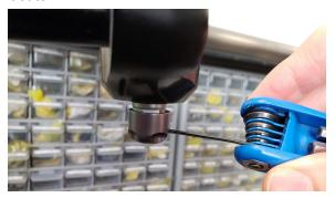
24. Apply a fresh drop of blue 243 loctite to the set screw and torque to 8in.lbs using a 1.5mm Allen key. Ensure the set screw is aligned so that it contacts the flat portion of the adjuster shaft.
