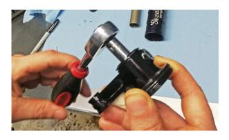
**2.8** Assemble Reservoir Inner Tube to Valve Housing.
