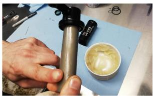
2.9 Apply Slickoleum/Slick Honey to IFP seals& assemble onto Inner Tube with the step side down.
