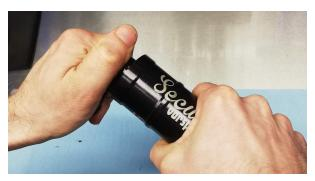
2.1 Remove Inner Tube and IFP by pushing Reservoir End Cap in until you can grasp one or both of the IFP and Inner Tube.
