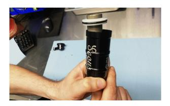
**2.2** The Secus standard service procedure typically entails replacement of dynamic (moving) seals and footstud outer seals only.
