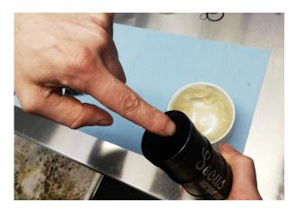
**2.12** Thread Reservoir Outer to Valve Housing by hand. Do not tighten fully yet.
