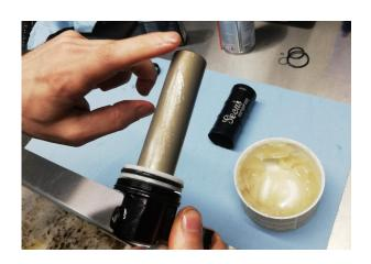
**2.11** Thoroughly clean Reservoir Outer. Inspect for damage.
