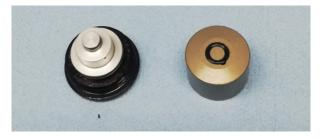
**2.4** Remove o-rings from IFP and Valve Inner.
