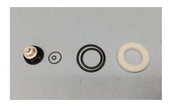
2.6 Apply oil (Float fluid or 20wt fork oil) liberally to the o-rings on the Valve Inner. Also lubricate the inner surface of the Valve Spool (do not get any excess oil in the centre hole/groove).
