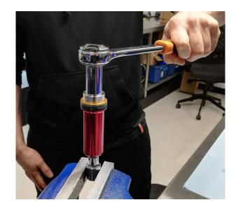
**1.10** Handscrew new piston base onto piston and place red loctite onto threads.
