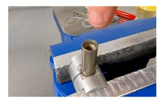
**1.5** Place a drop of red Loctite onto Secus footstud thread. Do not get any on the o-ring. Thread it down on to the shaft by hand
