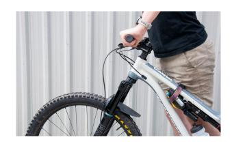
**3.3** Continue the process of adding more air & pushing down again to equalize the fork pressure to your desired pressure.
