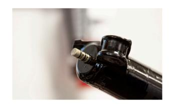
**1.15** Place installation tool over footstud & wind down nut. Use an 11mm socket to pull the shaft through until you feel minor resistance. Don't do it up tight. Remove installation tool.
