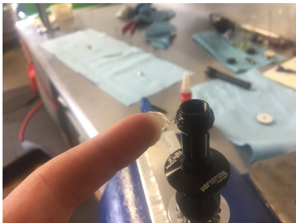
15. Grease the outer o-ring with Slick Honey
