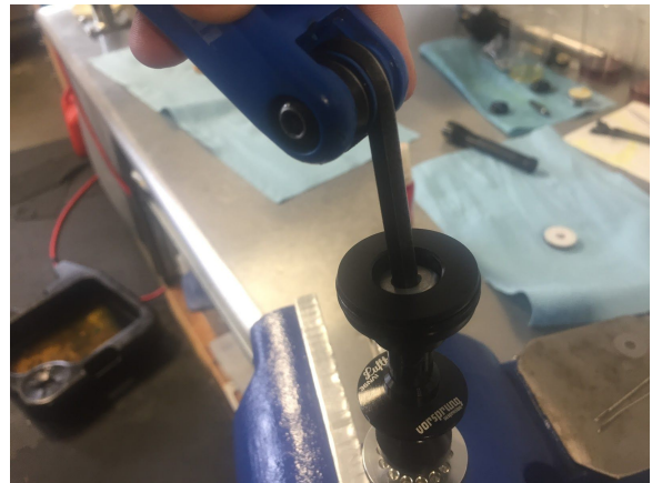
17. Apply red loctite to piston nut thread. Install piston nut into stud to clamp piston. Do not tighten by hand!
