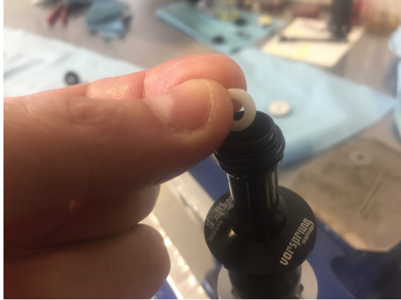
13. Install the second white backup ring above the o-ring.
