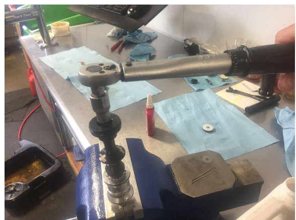
18. Use a torque wrench to torque piston nut to 50in.lbs. This will also torque the stud to the shaft - expect it to feel "soft", this is normal.
