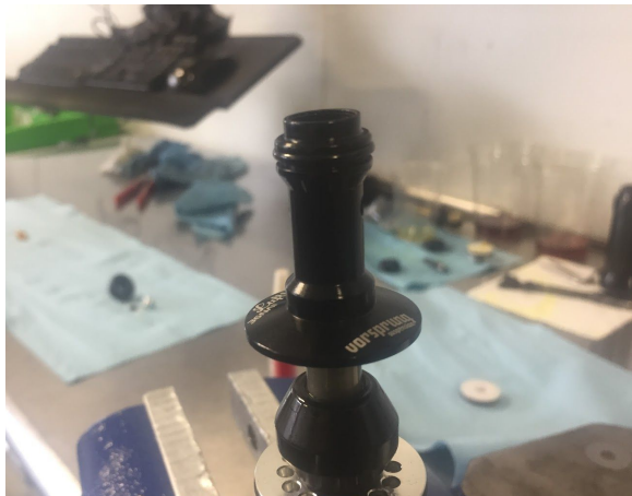
14. Install a new outer o-ring in the groove on the outside of the piston stud.
