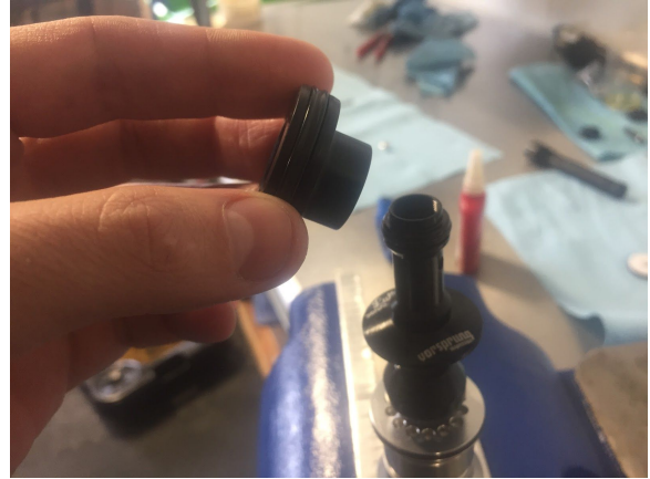
16. Install new black piston onto stud, wider end facing upwards
