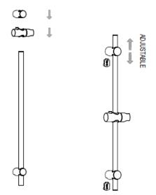
4. Attach hose to water supply elbow and hand shower. Fit the hand shower into slider bracket.
