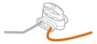
3. Press the connector firmly by using a pair of pliers
