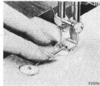
Fig. 74. Sewing Buttons with Thread Shank.
