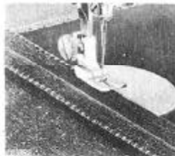
Fig. 65. Overedging Open Seams in Process.
