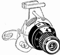
Needle thread tension too light — correct by setting dial to lower number.
