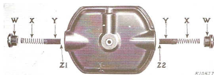
FIG. 17. BRUSHES READY FOR REPLACEMENT
