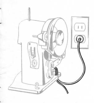
The SINGER\* Electric Motor in your sewing machine is furnished for operation on an alternating current of 110-120 volts, 25 to 75 cycles, or on 110-120 volts direct current.
