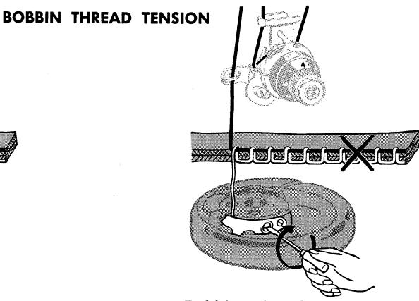
Bobbin thread tension too loose—correct by turning screw in direction indicated.
