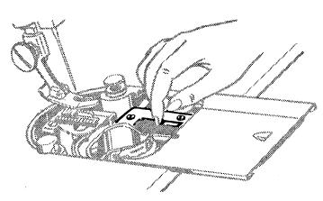
To clean hook raceway, remove bobbin case as follows—
