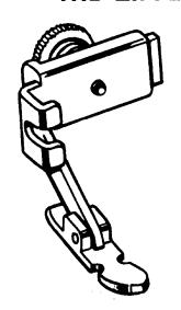
This foot is designed to facilitate the placement of stitching close to a raised edge. The hinged feature of this foot insures even feeding over pins, heavy layers of fabric or cross seams. It is attached to the machine in place of the regular presser foot, and may be adjusted to either the right or left side of the needle.
