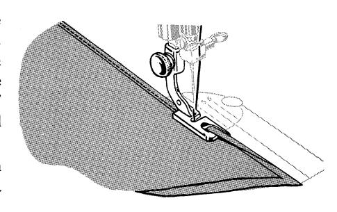
The seam may be stitched flatly to the garment, if a flat seam is desired. Open the work out flat, then insert the hem into the scroll. The hemmer will regulate the stitching uniformly from the edge of the hemmed seam.
