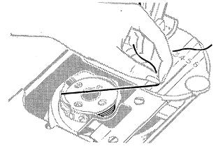
• Draw thread into notch at end of spring; pull about 3 inches of thread across bobbin.
