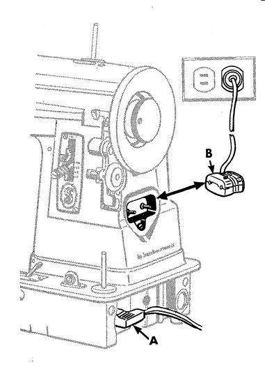
The SINGER\* Electric Motor in your sewing machine is furnished for operation on an alternating current of 110-120 volts, 25 to 75 cycles, or on 110-120 volts direct current. Special motors can be provided through your SINGER SEWING CENTER for direct or alternating current for any voltage between 50 and 145, and for 32 volts direct current.
