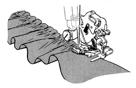
The length of the sewing machine stitch also affects ruffle fullness. Since a given attachment setting puts an equal amount of fullness into each stitch regardless of its length, shortening the stitch (more stitches to the inch)
