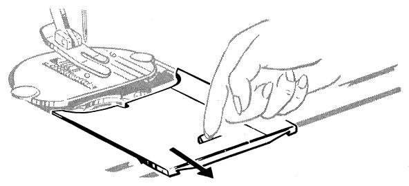
• Open slide plate and remove bobbin.
