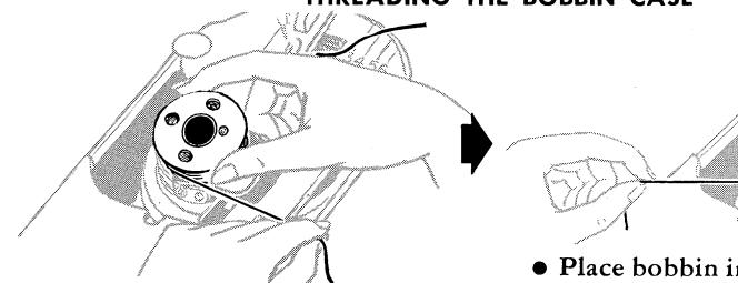
• Hold bobbin so that thread leads off in direction shown.
