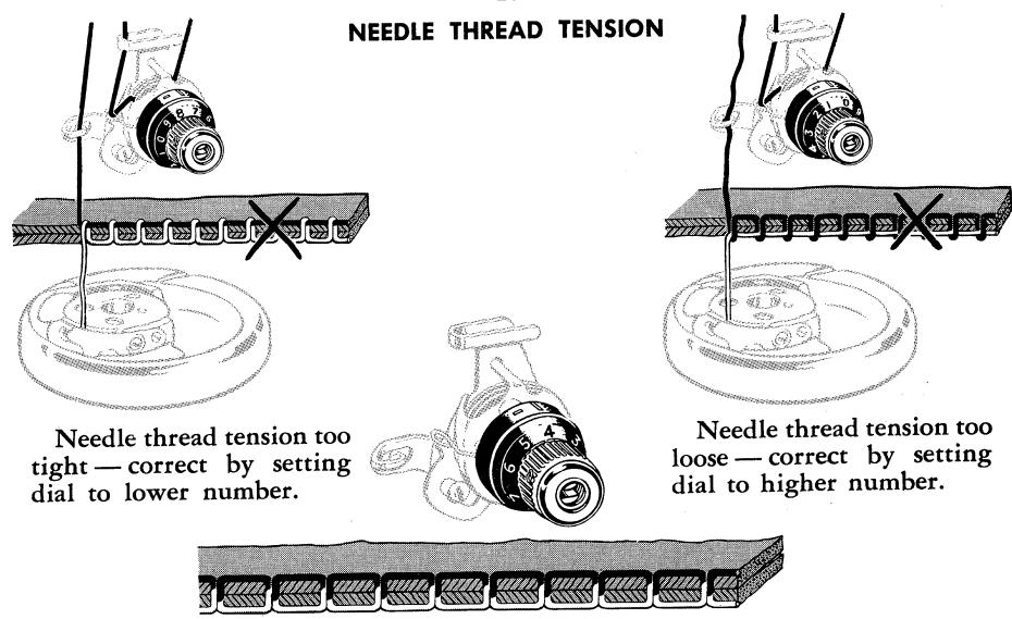
A perfectly locked stitch results with upper and lower tensions balanced so that needle and bobbin threads are drawn equally into fabric.
