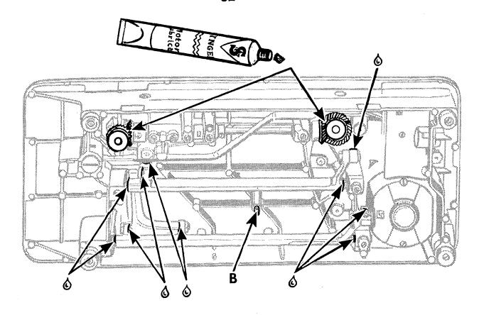
Tilt machine back and remove thumb nut from screw B, being careful not to lose felt washer, and remove cover from underside of machine.
