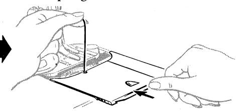
• Close slide plate allowing thread to enter notch.
