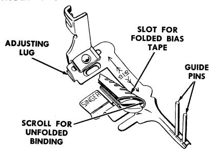
The multi-slotted binder is used to apply commercial binding as well as self fabric bias to an unfinished edge.
