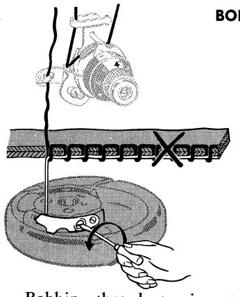
Bobbin thread tension too tight—correct by turning screw in direction indicated.
