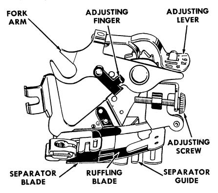
This attachment offers a simple and effective way to make gathered and pleated ruffles. Ruffles may be made separately or made and applied at the same time. The ruffler is attached to the presser bar in place of the regular presser foot.
