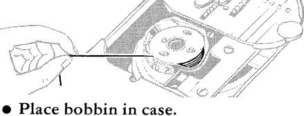
• Lead thread into slot and under spring.
