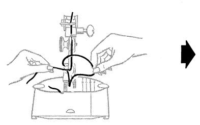
• Pull end of bobbin thread through plate.
