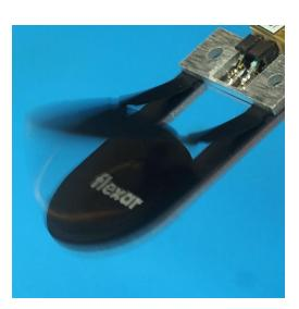
To control the motion of this actuator, one must use an h-bridge module, like the <u>Flexar Driver</u>. The magnetic field strength of this coil is limited to 2.7mT (measured from the surface). Given that some aspects of this actuator are customizable, its motion and force will also depend on the magnet's pivoting point and mass.
