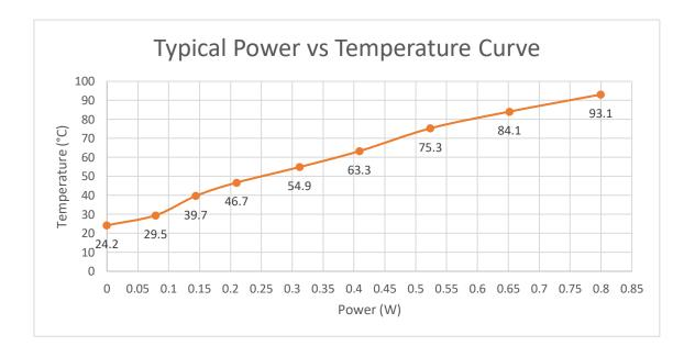
Please note that by driving the coil with a constant voltage will increase its temperature. This will also increase the resistance and thus lower the current flowing through the coil. This effect can be resolved by controlling the coil with a constant current driver.
