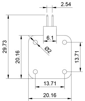
Please note that, the exposed copper on the PCB is used for heat dissipation. This must not be grounded or connected to any other signal. If connected to a signal, one might see a drop in the coil's magnetic field strength.
