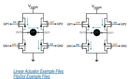
an h-bridge, such as the <u>Flexar</u> <u>Driver</u>. The image below shows an h-bridge circuit which can drive and control the current flowing through the windings.
