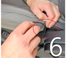
Drop the string closest to the door between the plastic trim and the seat cushion to run it on the inside of the seat frame.
