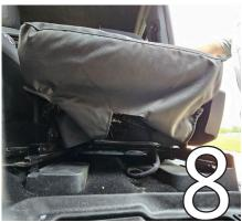
Run the long flaps under the seat to the back.
