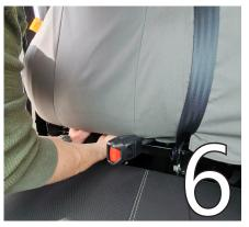
Next, wrap the tabs at the bottom of the seatback cover under the seat and secure behind it.
