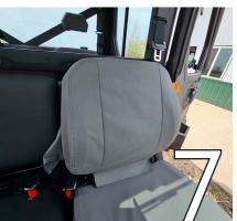
Undo all of the tabs for the seat back, and place it over the seat back.
