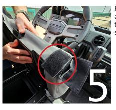
Fasten the upper and lower tabs tightly together at the back as shown.
