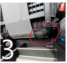
The headrest cover is the simplest piece! Just put it on and fasten the tabs underneath.
