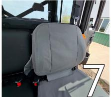
Undo all of the tabs for the seat back, and place it over the seat back.
