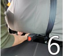
Next, wrap the tabs at the bottom of the seatback cover under the seat and secure behind it.
