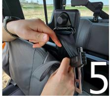
Having the 'soft' side of the tab facing the back of the cab makes this easier, so it doesn't stick on the way down.
