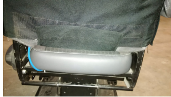
1.6- Fasten flap to back of seat
