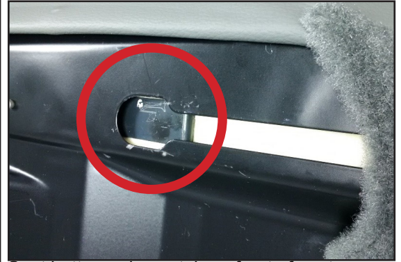
Seat bottom release tab on front of seat. Two per seat bottom.
