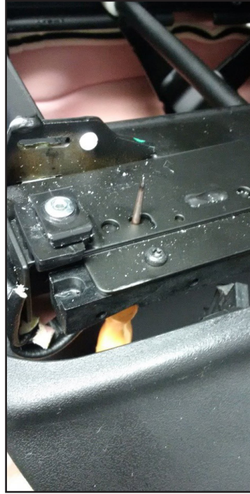
Seat bottom release tab on front of seat. Two per seat bottom.
