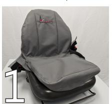
Pull the seat bottom cover around the seat bottom.
