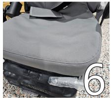
Place the seat bottom cover on. Watch out for the seat adjustment bar - make sure that is still exposed.
