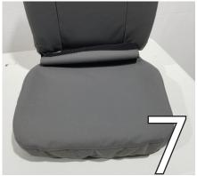
Place seat bottom cover over the seat bottom. Push flap between the back and bottom.
