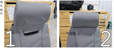
Tuck flap under the headrest and secure up inside the back of the headrest cover.
