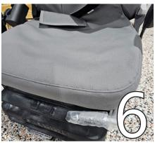
Place the seat bottom cover on. Watch out for the seat adjustment bar - make sure that is still exposed.
