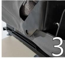
Run tabs around to the back of the seat, making sure they're under the metal brackets on the edge of the seat.
