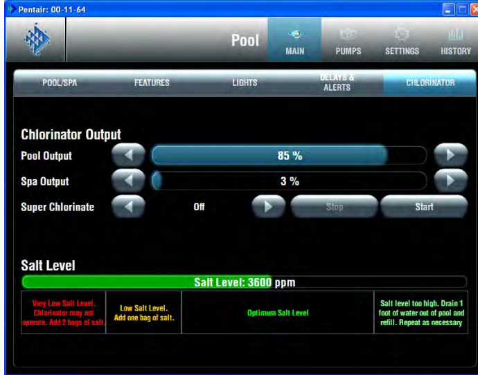
Chlorinator (IntelliChlor) screen
