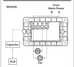
**Note:** The external capacitor forms part of the fan speed controller circuit. It is connected to the internal PCB and terminal A. Please make sure the wire connects to
