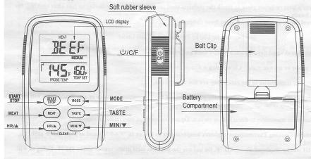
LCD (Liquid Crystal Display) – Displays all icons, temperature and timer. The backlight will flash Blue once the temperature increases 10F, will change to Green when the temperature is within 15F of the set temperature and will turn Red when it reaches the set temperature. See LCD diagram for detailed information.
