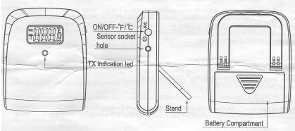
Stand - Fold up stand for easy storage. BATTERY COMPARTMENT - holds 2 AAA batteries (included).
