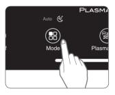
• When in Auto mode the fan speed is automatically adjusted according to the indoor air quality. As the indoor air quality improves, the fan speed will automatically be reduced. If the indoor air quality decreases, the fan speed will automatically increase.
