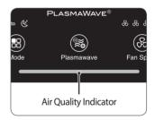
• Air quality level is displayed on the indicator, based on the Particle Sensors. Depending on the immediate environment, the indicator may change frequently in color or stay the same for lengthy periods of time.
