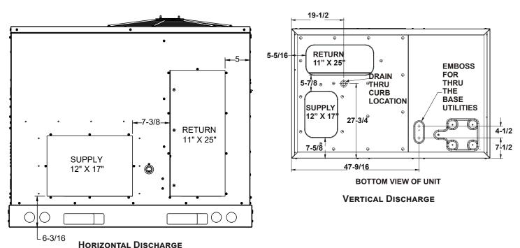
NOTE: REFER TO IOD-7082 INCLUDED IN THE LITERATURE PACK FOR INSTALLING HORIZONTAL DUCT COVERS.
