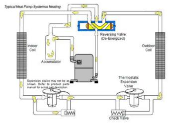
For Heat Pump units, the expansion devices are Fixed Thermal Expansion Devices (TXV) and perform the same function on the heating cycle as on the cooling cycle. The Fixed TXV also act as check valves to allow for the reverse of refrigerant flow.
