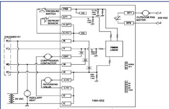
**DEFROST CONTROL WIRING SCHEMATIC**
