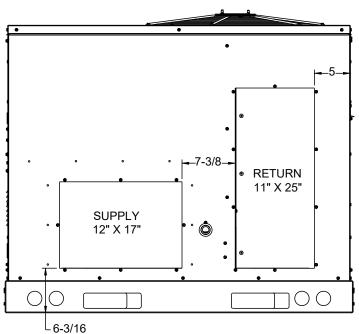
HORIZONTAL DISCHARGE DUCT CONNECTIONS
