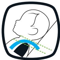
Rear-Facing (harness AT or just below shoulders)
