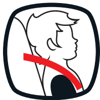
Forward-Facing (harness just above shoulders)
