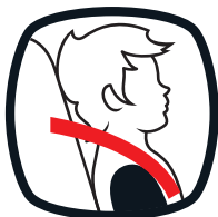
Forward-Facing (Harness just above shoulders)
