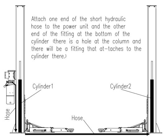
Run the long hose underneath the steel base plate as illustrated here and attach it to the hydraulic fitting at each cylinder.
