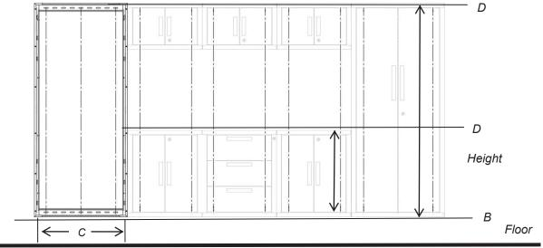
Note: Make sure that there are two studs to mount the locker on as it is easiest to start the installation with the locker first. Due to the spacing of the wall studs, some wall cabinets maybe have only one stud to attach to; this is acceptable if the wall cabinets are bolted together.
