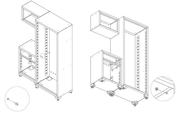
Repeat for the other locker and cabinets. Tighten all the bolts to fasten the cabinets and level the cabinets. The installation of the garage cabinet set is finished.
